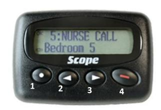
The pager is carried by the carer and will bleep or vibrate when it receives a signal from the transmitter, pressing **'4'** ACCEPTS the call and silences the pager. The pager has a working range of approx. 300m from the paging transmitter.
